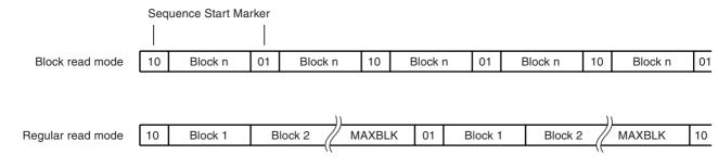
Figure 6-2. ATA5567 Sequence Start Marker in Extended Mode
