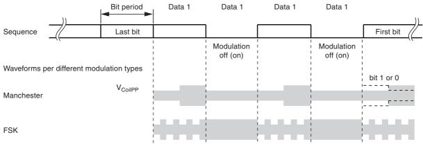
Sequence terminator not suitable for Bi-phase or PSK modulation
