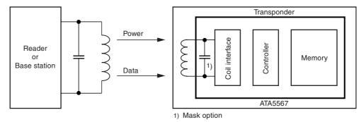
Figure 2-1. RFID System Using ATA5567 Tag
